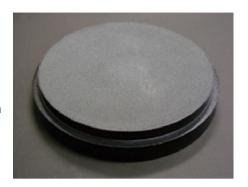
**Aluminum oxide** is the most standard material, with a density of 2.2 g/cc, and has a maximum operating temperature of 1400 F (800 C).
