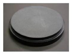
Aluminum oxide is the most standard material, with a density of 2.2 g/cc, and has a maximum operating temperature of 1400 F (800 C).
