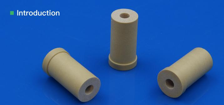
Magnesia Stabilized Zirconia (MSZ) is a great refractory and insulating material due to high oxygen ion conductivity, high strength and toughness, and good thermal shock resistance. It has a clean melt at temperatures above 1900°C and above and is specially manufactured for melting superalloys and precious metals. Its superior thermal shock resistance to temperatures reaching up to 2200°C.
